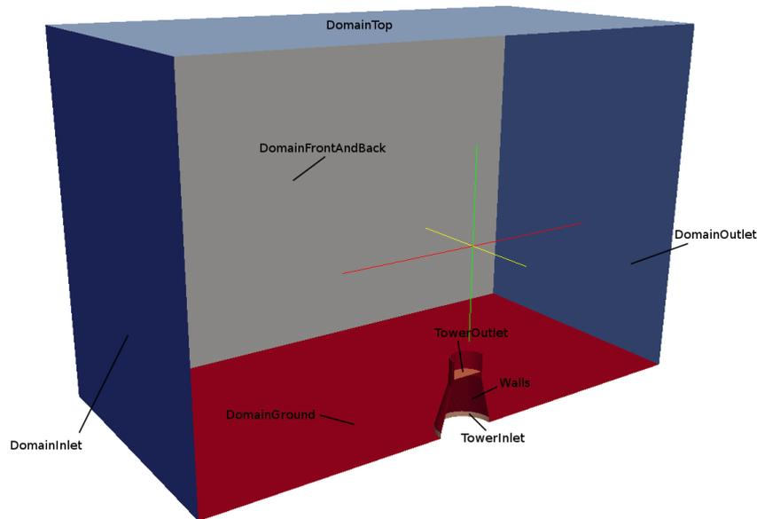
Figure 1 – definition of a simulation domain
