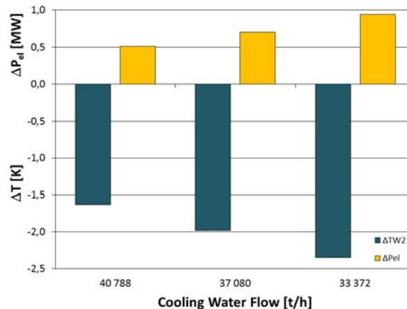
Figure 6: Effect of variation of cooling water mass flow on temperature level and power output
