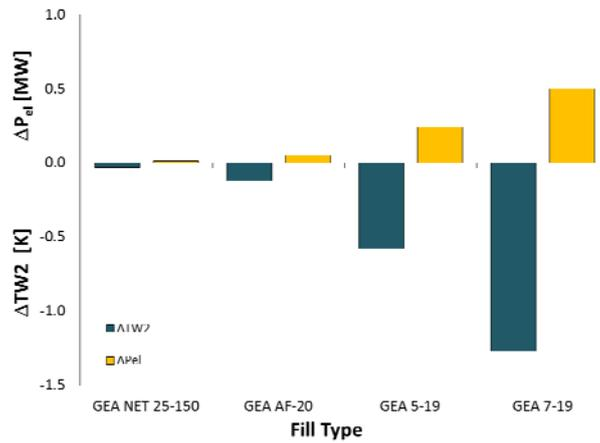
Figure 1: Thermal performance and power output for option 1 and different fill types
