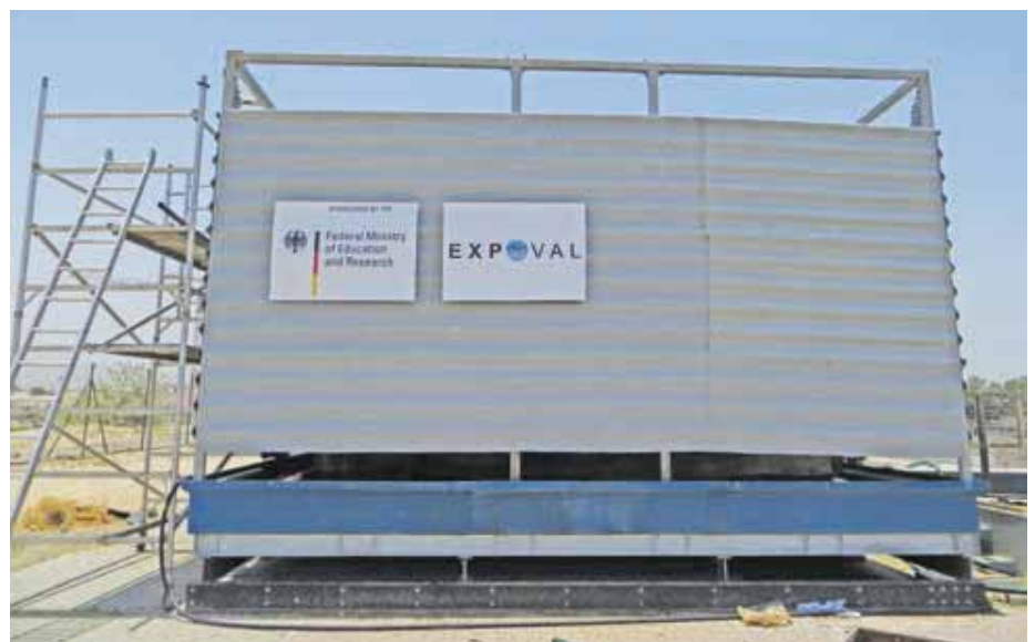
Right: Trickling filter pilot plant at Warsaw Sewage Treatment Plant in Dubai, United Arab Emirates.
