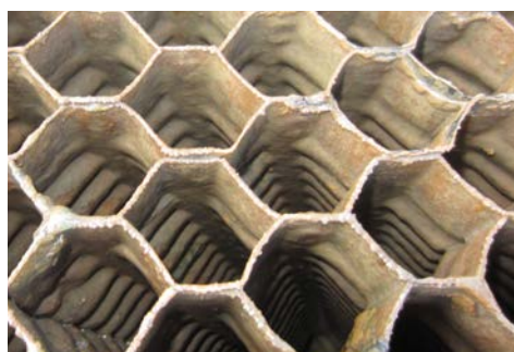
ODORdek packing with even distribution of biofilm
